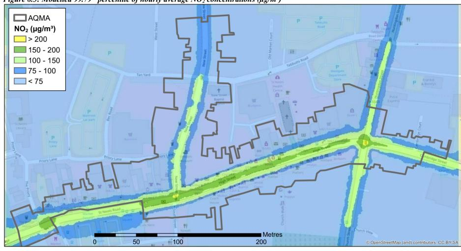
Figure 8.3: Modelled 99.79<sup>th</sup> percentile of hourly average NO<sub>2</sub> concentrations (µg/m³)
